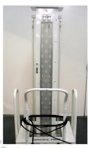
Test Device arrived in shipping crate. New UV bulbs were sent to replace damaged bulbs. UVC dosage labels, and device remote were also included with device.
