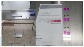
Left: Test carriers are held in place on tray for treatment. Photo shows carriers facing device at floor height and 3 feet. Carriers 5 feet from test device.
